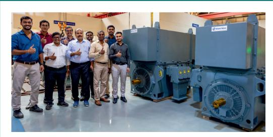
Our Closed Air Circuit Air-Cooled (CACA, IC611) medium-voltage motors feature a robust, enclosed cooling system, ensuring optimal performance even in heavy-duty applications and demanding environments. These motors have excelled in third-party inspections, and the batch pictured here was delivered to Madhya Pradesh Jal Nigam (MPJN).
