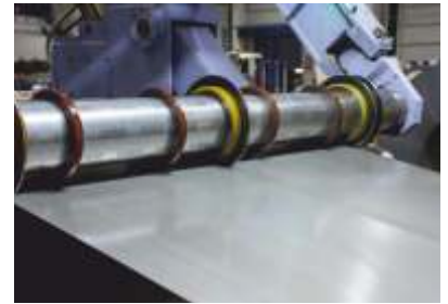
Continuous shear control for CTL in rolling mill
